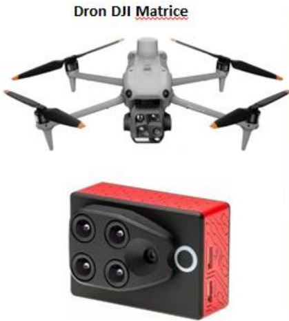
Sensor RGB oraz cztery kanały spektralne: Green (550 nm), Red (660 nm), Red Edge (735 nm), Near infrared (790 nm).
